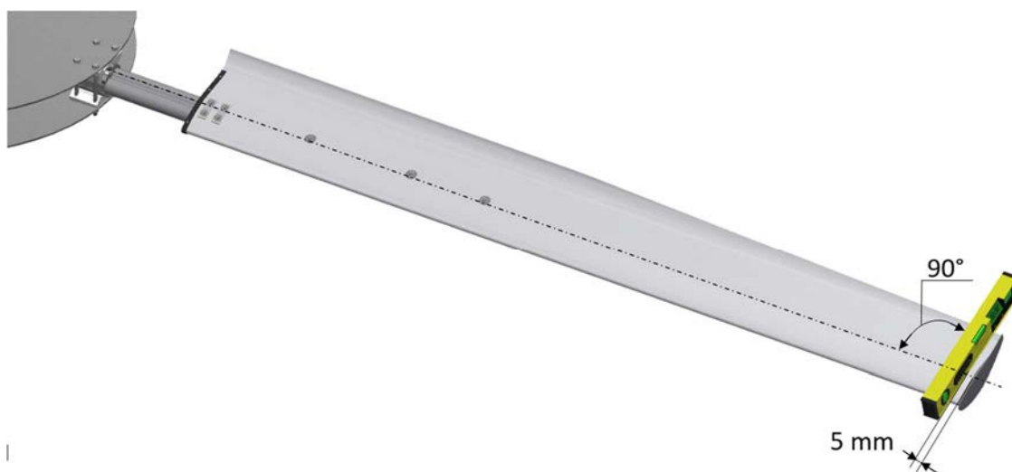
Figure 2.19: positioning of protractor on blade
