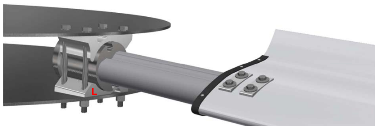
Figure 2.18b: blade installation on hub: mounted
